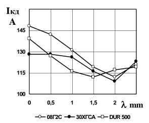
Fig.4. Impact of the amplitude of vibrations  $(\lambda)$  on the amperage at the end of arc combustion (length of arc combustion) during vibroarc weld overlay in Ar with different wire electrodes
