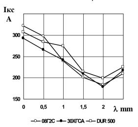
Fig.3. Impact of the amplitude of vibrations  $(\lambda)$  on the short circuit amperage (I short circuit) during vibroarc weld overlay in Ar with different wire electrodes
