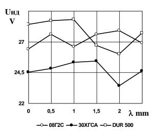
Fig.2 Impact of the amplitude of vibrations  $(\lambda)$  on the voltage at the start of arc combustion (U start of arc combustion) during vibroarc weld overlay in Ar with different wire electrodes
