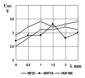
Fig.1. Impact of the amplitude of vibrations  $(\lambda)$  on the short circuit voltage (U short circuit) during vibroarc weld overlay in Ar with different electrode wires
